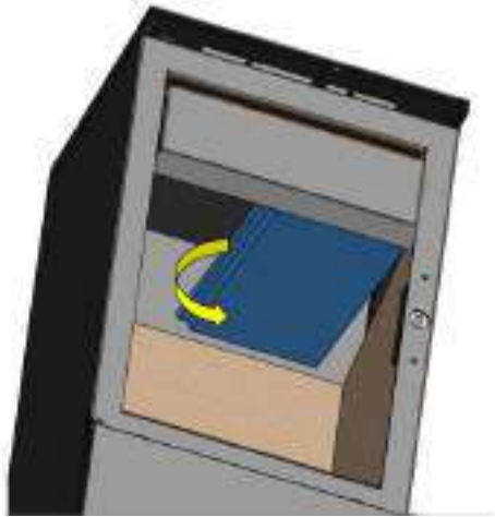
Figure No.7 - Extracting the vermiculite deflectors
